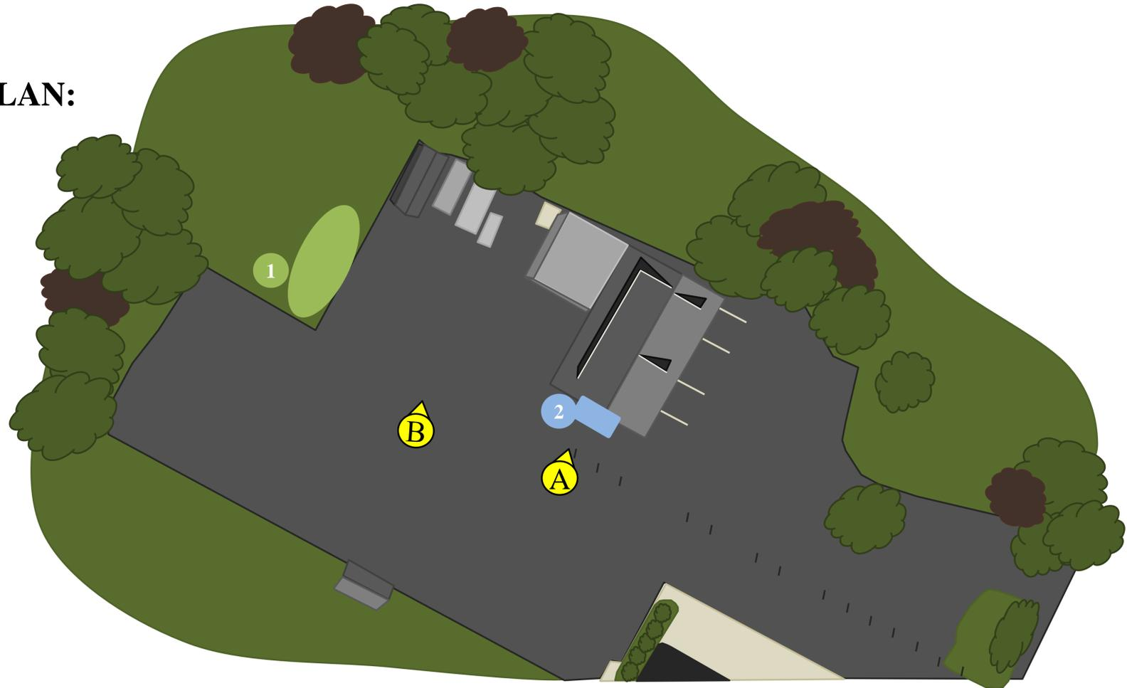
**1 BIORETENTION SYSTEM:** A bioretention system could be installed in the grass area towards the back of the parking lot to manage stormwater runoff from the parking lot. A bioretention system will reduce runoff and allow stormwater infiltration, decreasing the amount of contaminants reaching catch basins.
