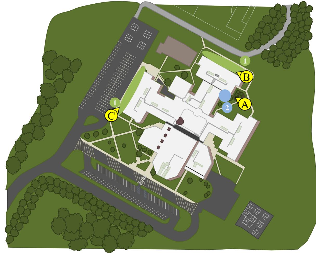
**1 BIORETENTION SYSTEM:** Bioretention systems could be installed along the sides of the school after disconnecting several downspouts. Bioretention systems will reduce runoff and allow stormwater infiltration, decreasing the amount of contaminants reaching catch basins.
